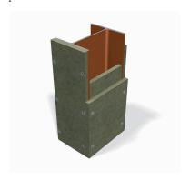
**2** Press the pieces of insulation between the flanges behind a coming joint.
